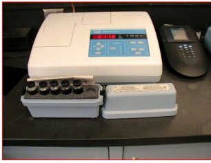
Bench-top Turbidimeter & Primary Standards
